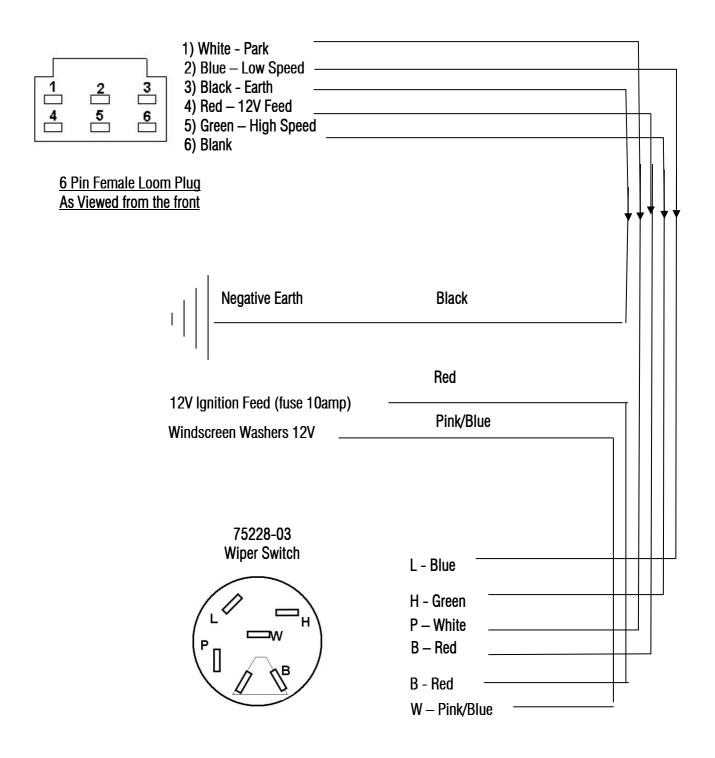
Wiper switch system is 12V Positive Feed
